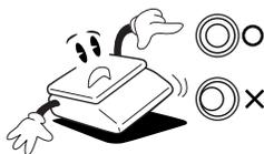
By adjusting 4 comers of the scale, set the scale even using the built in scale leveling indicator.
